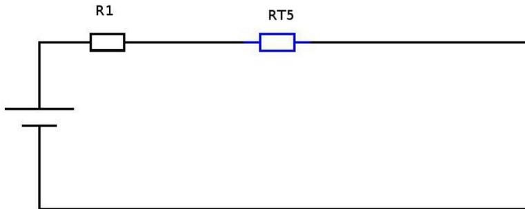
$$\begin{aligned} RT &= R1 + RT5 = \\ &6 + 1,5 = \\ &7,5 \Omega \end{aligned}$$
